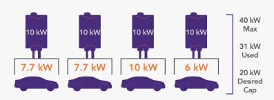
**With load balancing,** the maximum load is set at 20 kW. All four cars charge below their individual acceptance rates, making it easier to limit the overall consumption and manage demand charges.
