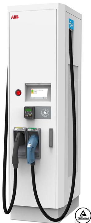
Building off a decade of EV fast charging experience, ABB's Terra 54 joins the Terra family of bestselling DC fast charging stations for enhanced usability and reliability. The Terra 54 enables continuous 50 kW charging up to 500V, while 200 – 920 V is supported by Terra 54HV.
